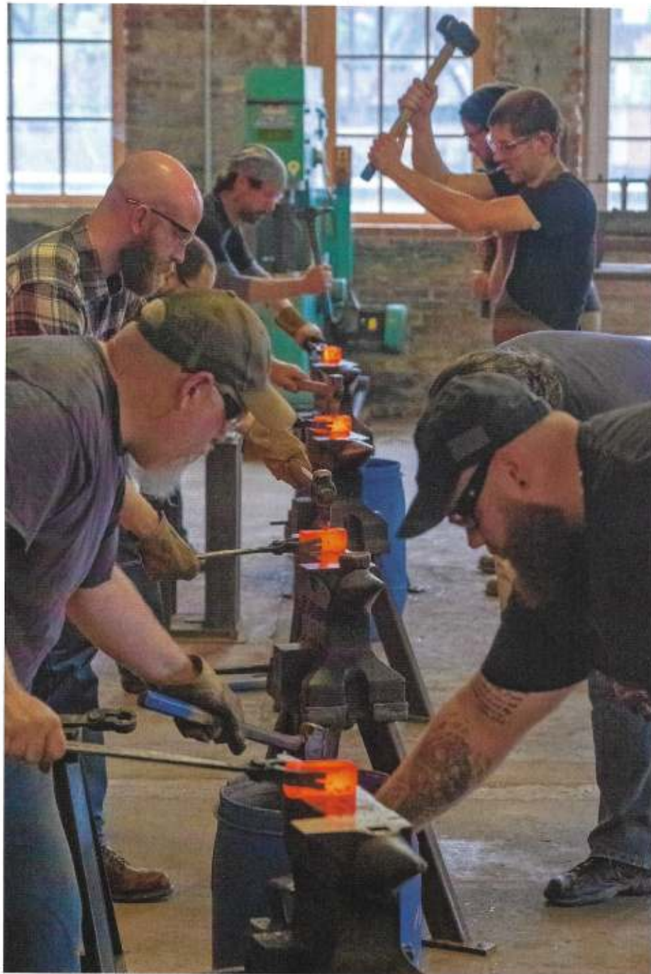
Students work with each other to strike punches in chunks of tool steel and create the eye in hammer heads (for the handles) during a workshop in October 2018, the first year that the school held classes in the shops in Johnstown.
